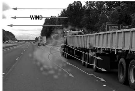
A crosswind pushes the bow wave of air around the front of a truck to the downwind side.
